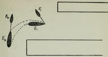
E<sub>1</sub> "Edith" reversing and backing to her starboard eases strain and assists F<sub>1</sub> "Fearless" in swinging head around with minimum strain on towing hawser.
